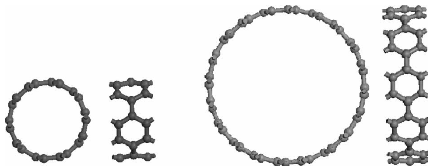
Figure 1. (a). (5,5) SWNT—20 atoms (b). (10,10) SWNT—40 atoms.
